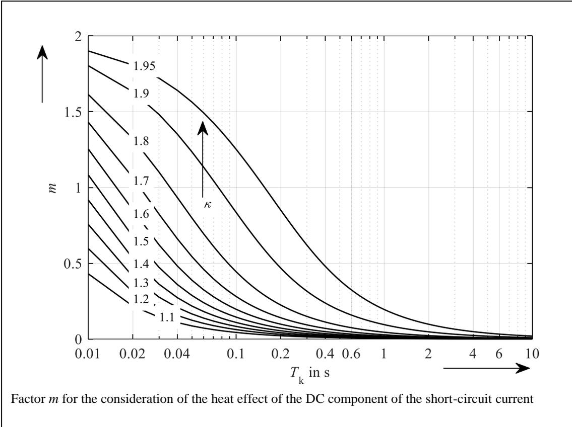
Factor  $m$  for the consideration of the heat effect of the DC component of the short-circuit current
