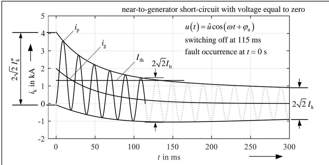
$$i_k(t) \approx \sqrt{2} \left[ (I_k'' - I_k') e^{-\frac{t}{T_d''}} + (I_k' - I_k) e^{-\frac{t}{T_d'}} + I_k \right] \cos(\omega t + \alpha) - \sqrt{2} I_k'' \cos \alpha e^{-\frac{t}{T_g}}$$
