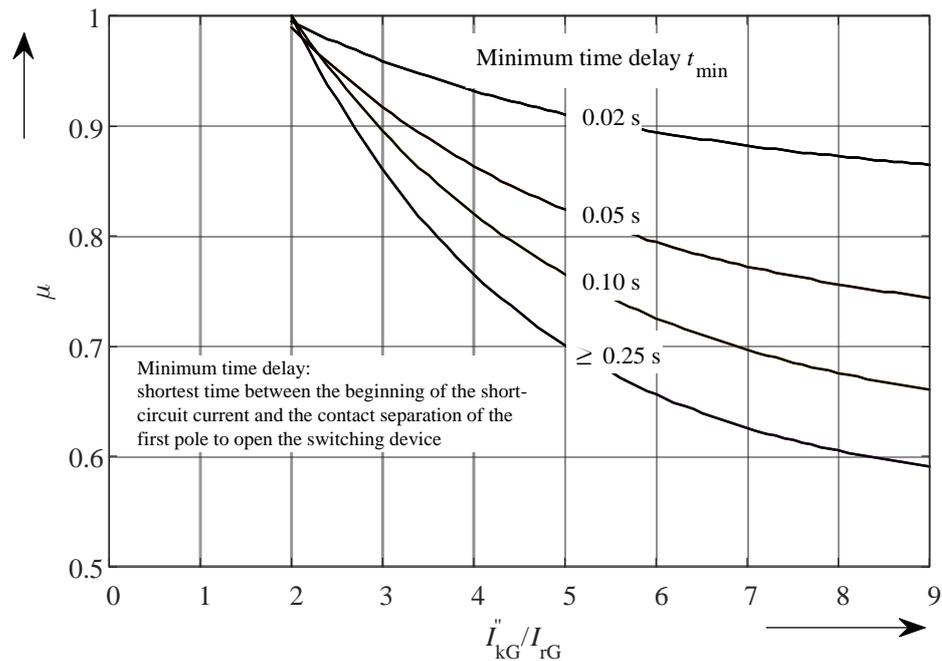
Factor  $\mu$  for the calculation of the symmetrical breaking current in case of a near-to-generator single-fed three-phase short-circuit
