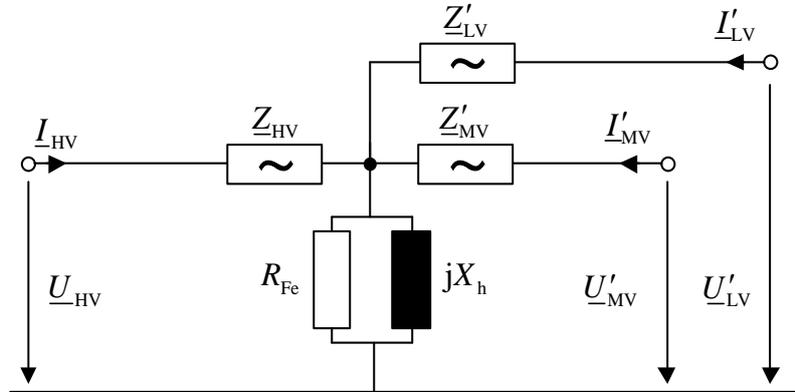
The calculation of the equivalent circuit parameters of a three-winding transformer is subject to the same calculation specifications as for the two-winding transformer. A minimum of three short-circuit tests is required to calculate the three series impedances. The magnetizing impedance ( $X_h$  and  $R_{Fe}$ ) is calculated according to Section 7.4.2 using the data of the open-circuit test.
