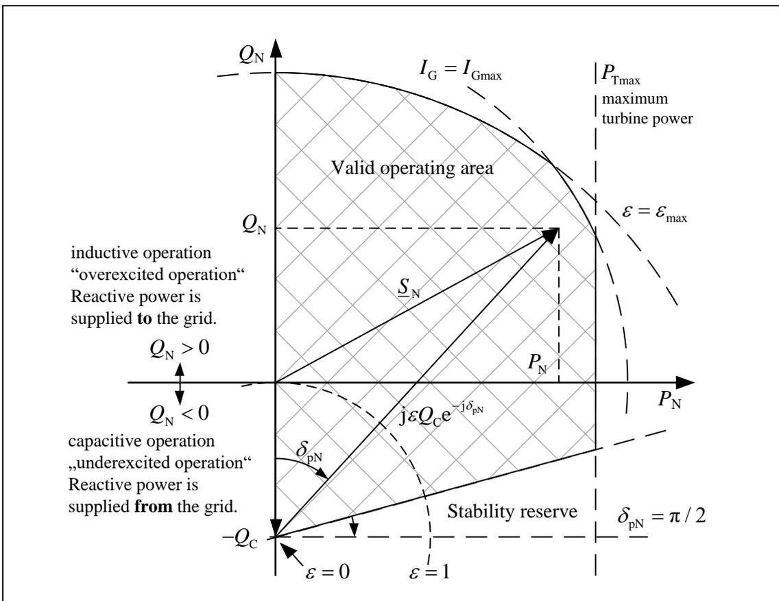
In practice, the operating ranges inductive and capacitive operation are also referred to as "overexcited operation" and "underexcited operation", although, depending on the current delivered to the grid, capacitive operation with  $Q_N < 0$  is also possible in overexcited operation of the synchronous machine with  $I_f > I_{f0}$ .
