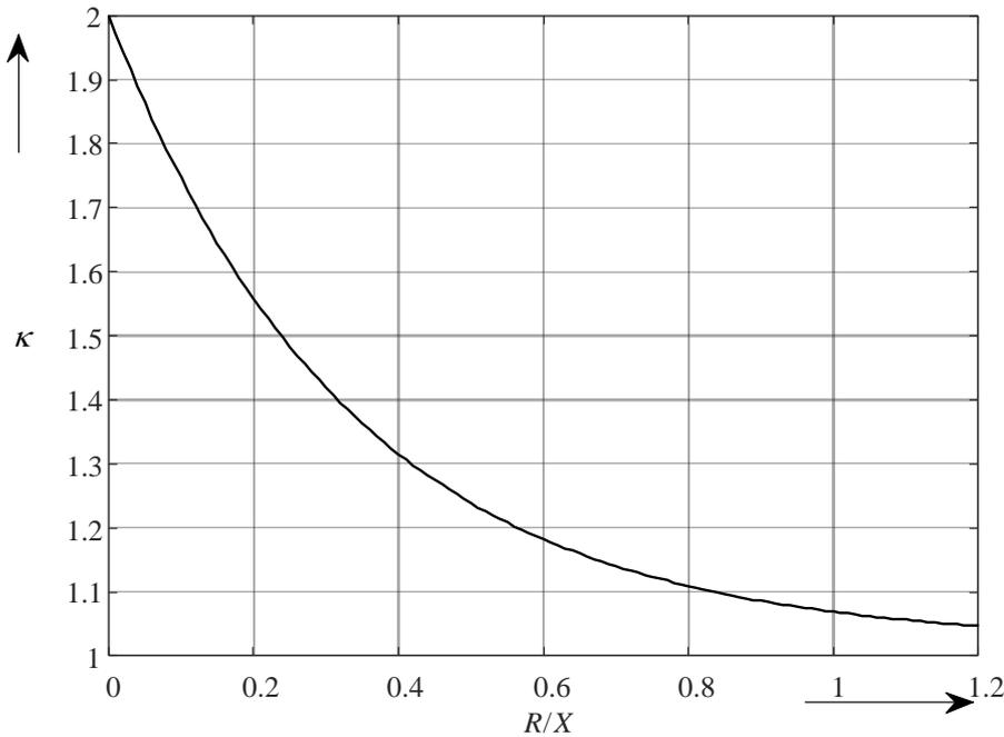
Factor  $\kappa$  for the calculation of the peak short-circuit current.
