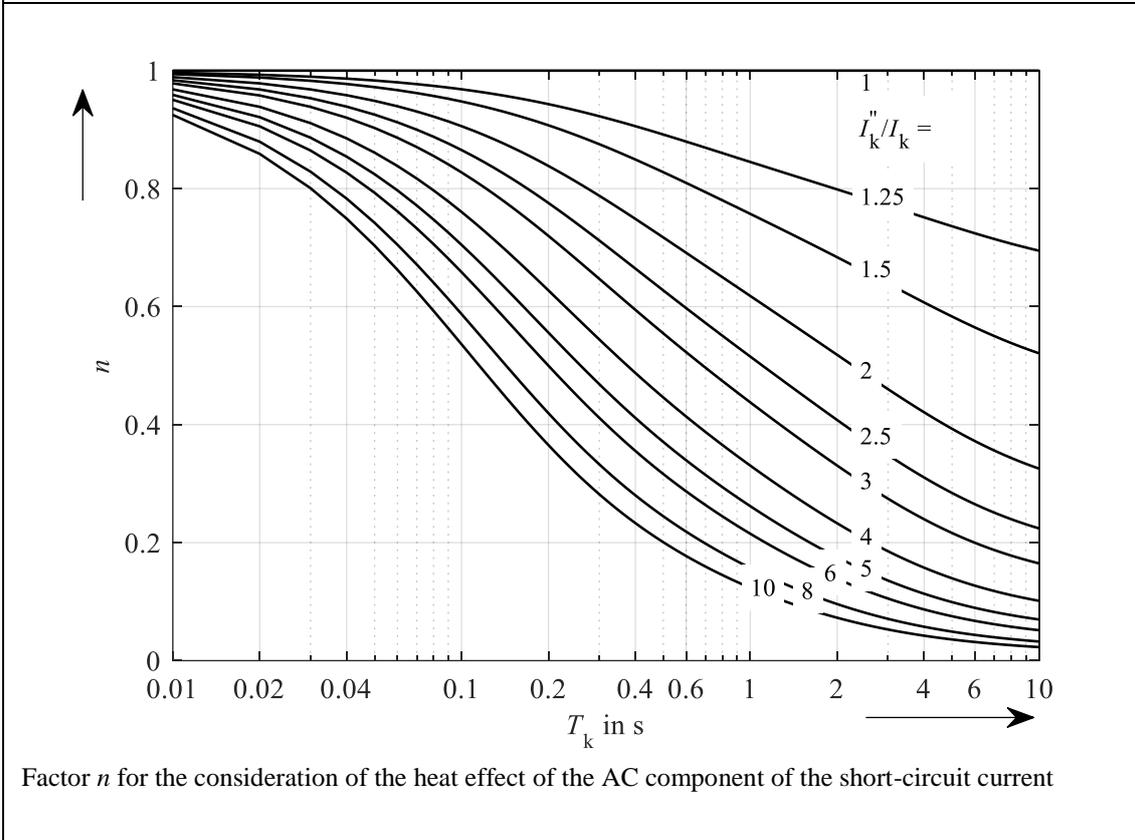
Factor  $n$  for the consideration of the heat effect of the AC component of the short-circuit current
