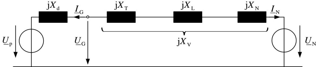
with the synchronous generated voltage  $\underline{U}_p = U_p e^{j\varphi_{Up}}$  and the internal grid voltage<sup>4)</sup>  $\underline{U}_N = U_N e^{j\varphi_{UN}}$
