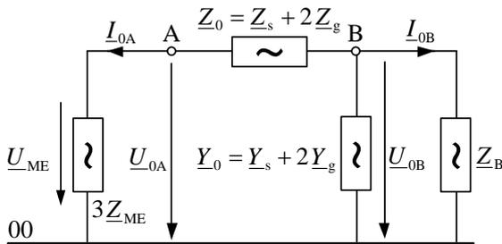
The neutral-to-ground impedance  $\underline{Z}_{ME}$  affects only the zero-sequence system. The neutral-to-ground voltage is:  $\underline{U}_{ME} = 3\underline{Z}_{ME} \underline{I}_{0A}$
