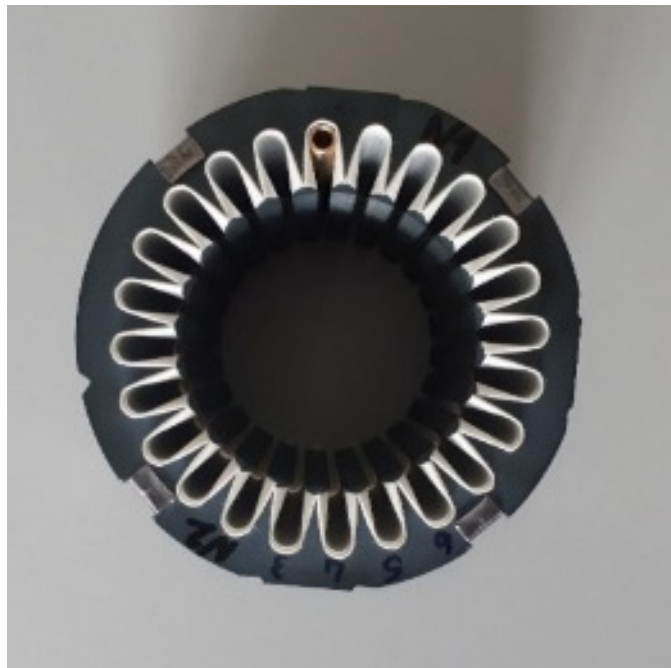
Figure 1: Stator with metal tube as counter electrode
