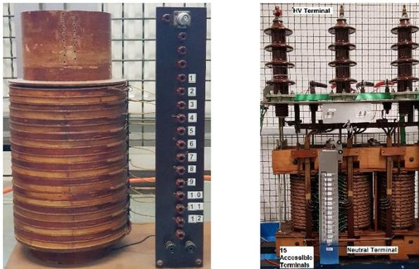
**Figure 2:** Two test objects; left: Model winding, right: 3-phase distribution transformer
