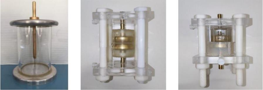
**Figure 2:** PD models for corona discharge (left), internal discharge (middle), and surface discharge (right)
